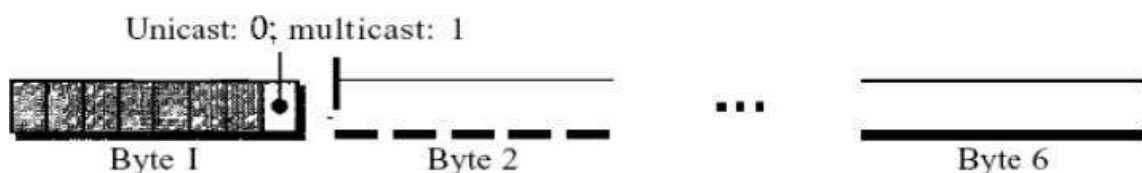
Figure 5 Unicast and multicast addresses
